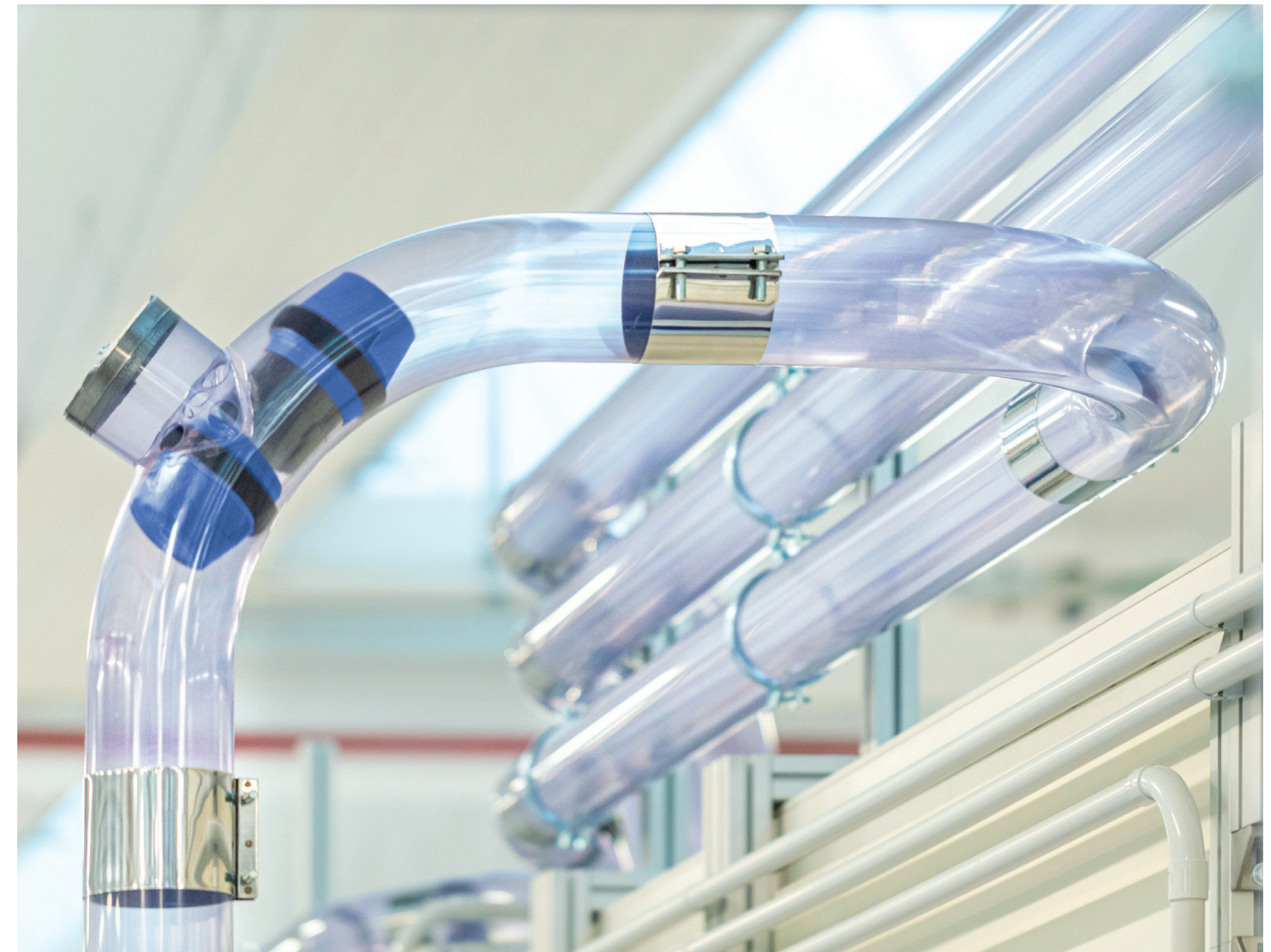
A transportation module that moves FFPE blocks from embedding to microtomy and final archiving.
